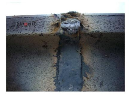
Last layers surfaced with hard wire.
