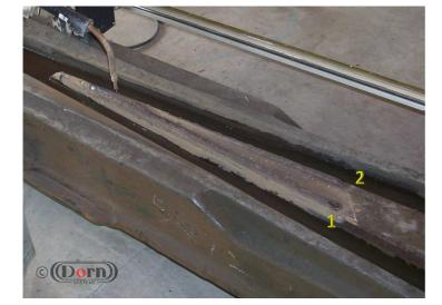
Multi Area welds with automatic count-down timer for "cold" rail.
